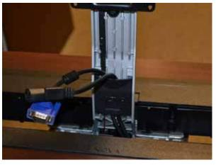
**Step 9**: Secure the monitor cables to clips located on either side of the modesty compartment and route the cable through grommets to the power strip and CPU shelf.
