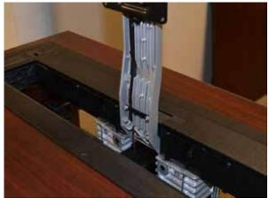
Step 6: Remove the right screw securing the strain relief and rotate the plate up as shown below.
