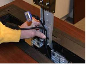
Step 8: Secure the strain relief over the monitor cables and re-attach the protective cover.
