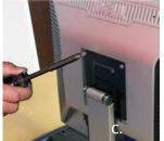
2c. Attach monitor to VESA plate using the four removed monitor screws.
